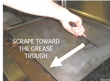
Figure 10: Remove scrubbing water
