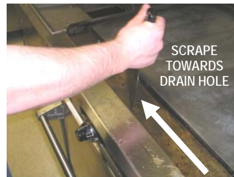
Figure 11: Clearing the grease trough
