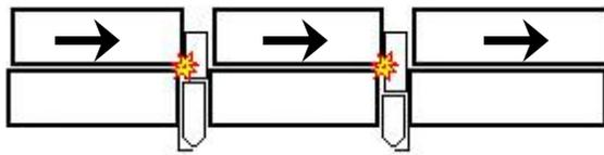
When the top plate is shifted to the left or the right it cannot move because, at the shear line between the two plates, the driver pins bind.
